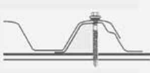
Crest fixing for roof or walls
